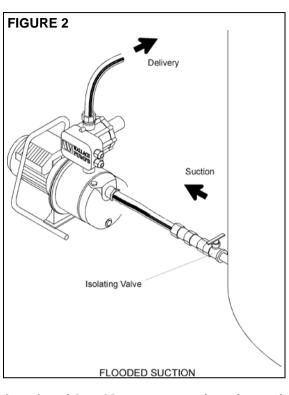
flooded suction piping. These pumps must not be directly connected to a pressurised suction. For boosting town supply install a 200 litre tank ( or larger if needed ) with a full flow ball cock from the town supply. Connect the pump suction pipe to the tank as previously described.
