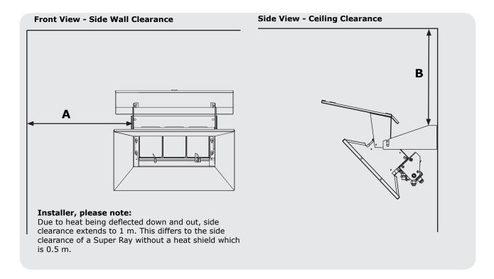
Angle of deflector is fixed and must not be altered. This is a safety feature.
