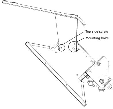
Front View of Fitted Heat Shield
