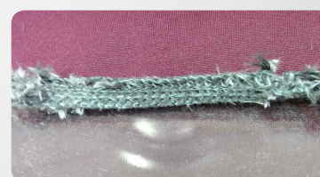
Example of a damaged glass seal
