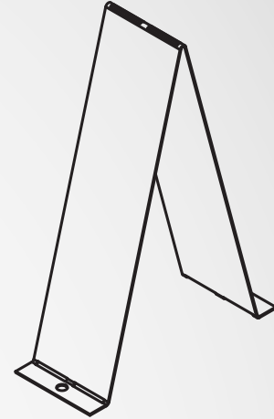
Step 2: Bend and secure metal standoffs
