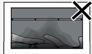
Soot build up
