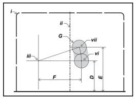
5. From the arc axis *iii* use the measurements *F*, *D* & *E* from **Table**1. to draw an arc on the wall.
