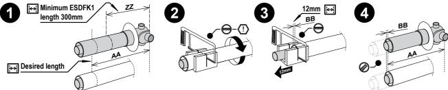
1. He Measure and mark off the outer pipe at the desired length (AA).
