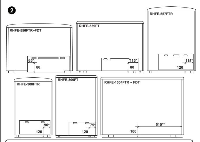
All vertical measurements are from floor level.
