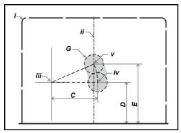
4. From the arc axis *iii* use the measurements *C*, *D* & *E* from **Table**1. to draw an arc on the wall.
