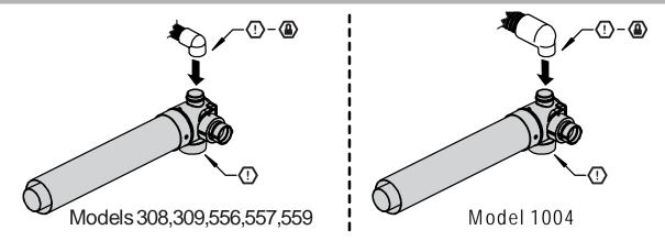
The combustion air hose of all Energysaver heaters is attached to the small diameter combustion air inlet.
