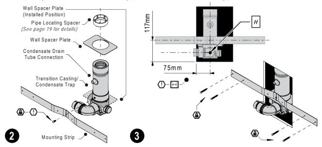
Using the screw removed from the front of the transition casting attach the mounting strip across the front of the transition casting.
