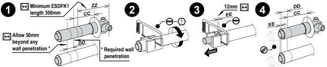
1. Measure and mark off the outer pipe at a point flush with the surface of the wall penetrated (**CC**) PLUS an additional 50mm (**DD**).
