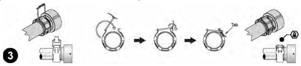
Close the clamp until the tab locks to secure both components together.
