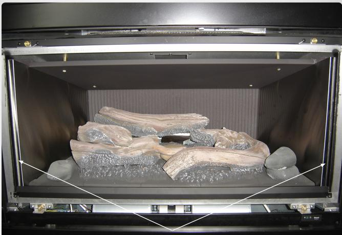
Reflective panels correctly positioned with return fold on top of the air guide, and back face of angled front edge meeting the front face of the ceramic panels.
