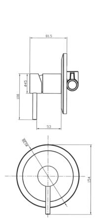
CARTRIDGE TYPE: Ceramic CLASSIFICATION: Suitable for mains pressure only INLET CONNECTIONS: 1/2 " BSP female OUTLET CONNECTIONS: 1/2 " BSP female WORKING PRESSURE: 150 - 500kPa DIMENSIONS FOR FITTING: -OPERATING TEMPERATURE: 5 °C - 80 °C
