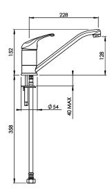
**CONSTRUCTION**: Brass body **CARTRIDGE TYPE**: Ceramic
