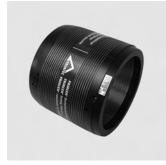
With exposed heating coils for optimal heat transfer, large insertion depth, wide fusion zones plus cold zones at the end and in the middle to prevent the flow of molten material, for use without holding devices. From d 180 with fusion indicators for visual fusion control.
