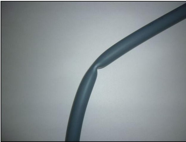
Figure 2 – Pipe Failure due to Kinking
