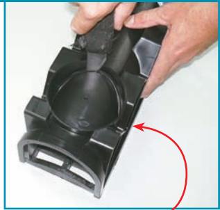
Cut or Drill 90mm bottom outlet.
