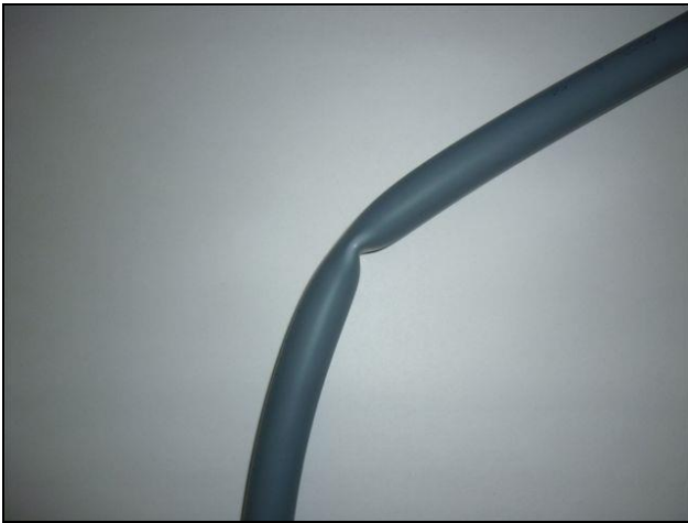
Figure 2 – Pipe Failure due to Kinking
