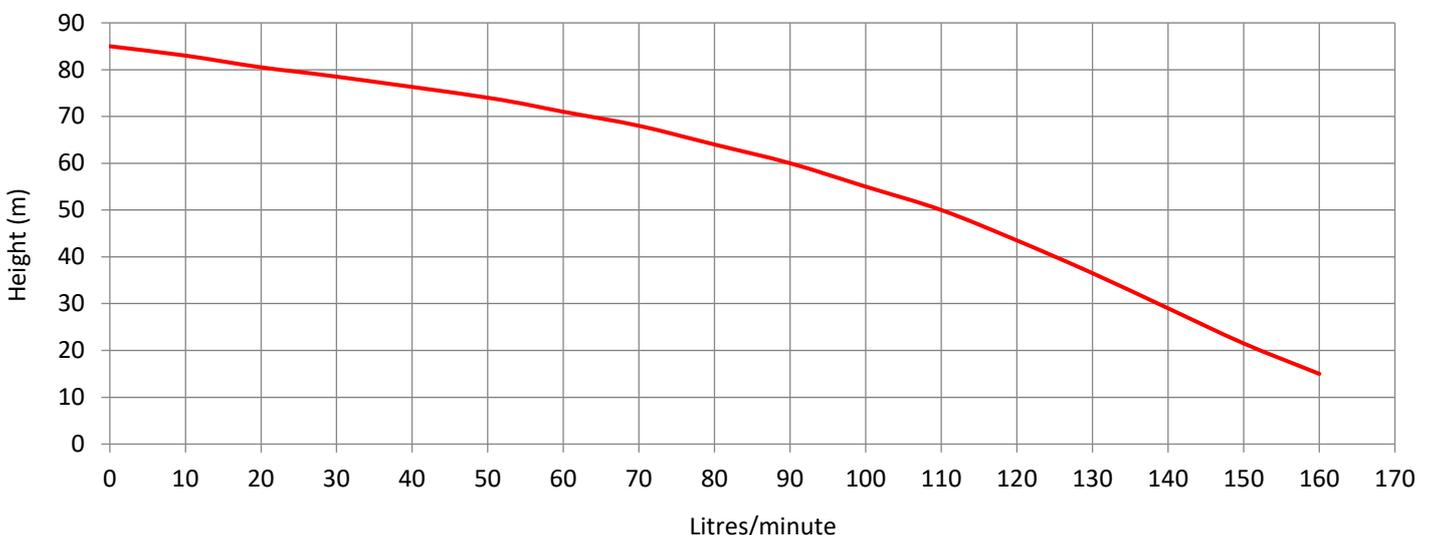
**NOTE:** The above Performance graph is measured at pump outlet and based on factory test conditions. Actual performance onsite may differ due to piping and fixture sizing and layout
