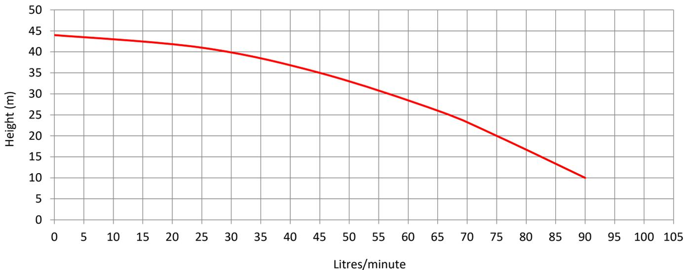
**NOTE:** The above Performance graph is measured at pump outlet and based on factory test conditions. Actual performance onsite may differ due to piping and fixture sizing and layout
