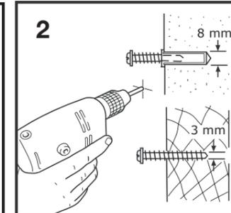
2 In masonry, drill 8mm diameter holes and insert the plugs provided. In timber, drill 3mm diameter pilot holes.
