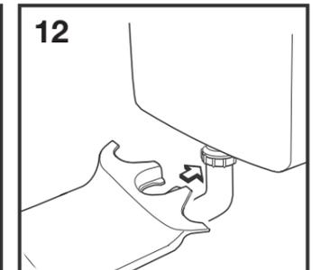
12 Push the link plate into position for marking.
