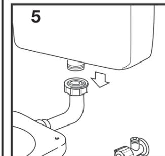
5 Lower the cistern onto the pipe and hook it over the mounting screws.
