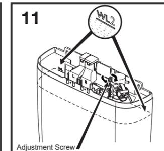
11 Actuate the Inlet valve at least once to purge any trapped air in the valve. Adjust the water level to the WL2 mark.
