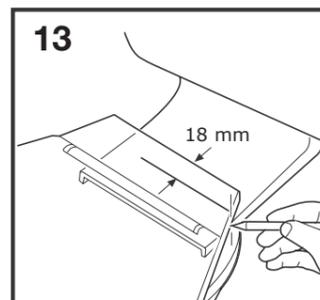
13 Position the seat and mark the link plate as shown.
