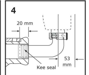
4 Cut the flush pipe to dimensions shown. Lubricate the kee seal with soap and water and fit the pipe into the pan. Fit the coupling nut and seal onto the flushpipe.
