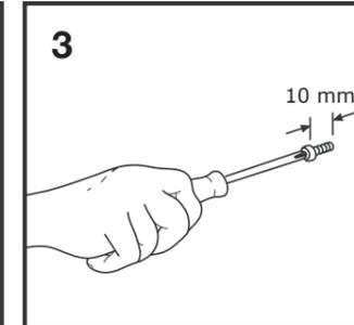
3 Leave the screws protruding by 10mm.
