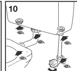
10 Turn on the water. Operate the cistern and check for leaks.
