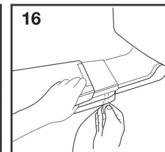
16 Tighten seat bolt nuts.
