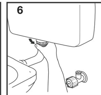
6 Hand tighten the coupling nut.
