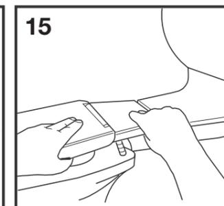
15 Push the link plate back into place and seat bolts into pan holes.
