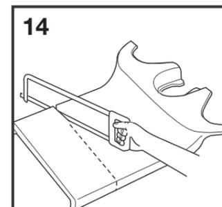
14 Fitting of the seat will be made easier if a sharp knife is used to put a bevel on the cut edge.
